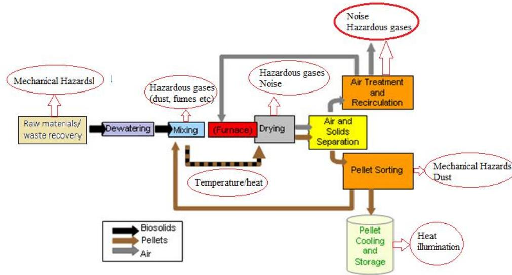
**Figure 1:** Potential Hazards From Different Fertilizer Manufacturing Processes
