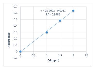
Figure 3: Calibration Curve for Cadmium
