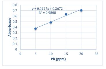
Figure 2: Calibration Plot of Lead
